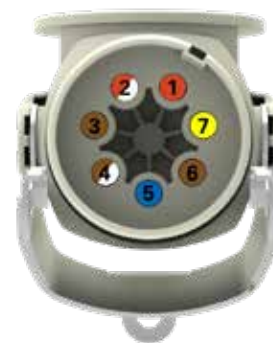
Steckbild des 7-poligen Steckers nach ISO 25981 Contact allocation of the 7-pin plug according to ISO 25981 with color coding
